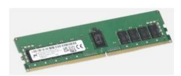
16GB Micron, 2Rx8, CL22, DDR4-3200Mhz, PC4-25600, 1.2V, RDIMM ECC Server Memory RAM
