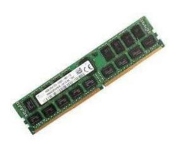
32GB SK Hynix, DDR4-3200Mhz, RDIMM 2Rx8, PC4-25600R, 1.2V, Dual Rank ECC Registered Memory Module
