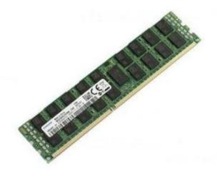
32GB Samsung, DDR3 PC3-12800R (1600MHz), ECC Registered RDIMM, Server Memory Module
