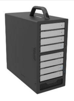
8-Bay Stardom SohoTank, 2x MiniSAS 6G/12G, 8x3.5 /2.5 SAS/SATA HDD/SSD, Removable **Drive Tray, Built-in Power** Supply, High **Performance Speed External Storage Enclosure**
