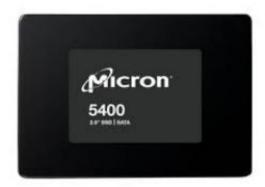
1.92TB Micron, **SATA, 6Gbs, 2.5,** 7mm, 5400 Pro **Enterprise** (non Sed) 176-layer, 3D TLC, **Sequential Read** (mbs) in 540 Mbs, Sequential Write (mbs) 520 Mbs Rand Read, 95000 IOPS, **Rand Write IOPS** 33000, 1.5 DWPD, SSD
